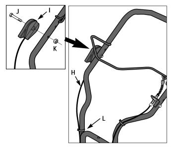
Figure 2-3: Attach throttle lever to right-side handlebar.
